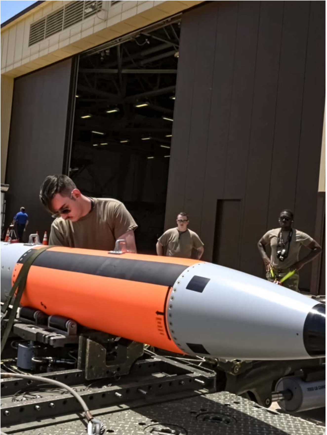
PHOTO 3: A non-nuclear mock B61-12 Joint Test Assembly (JTA) being prepared for test load for the B-2 Spirit bomber (U.S. Air Force photo by Airman 1st Class Devan Halstead)
